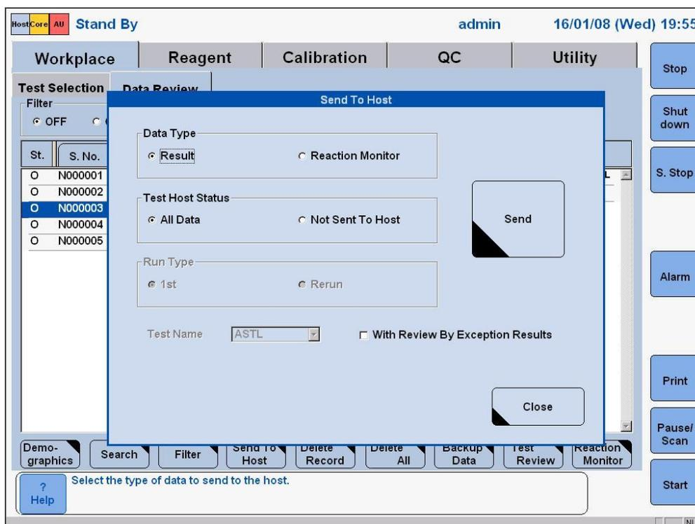
Note: Communication of batch results is based on option of “with Review by Exception Results” on [Send to Host] window shown below.
