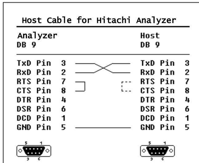
Fig. B-2 Connection Diagram
