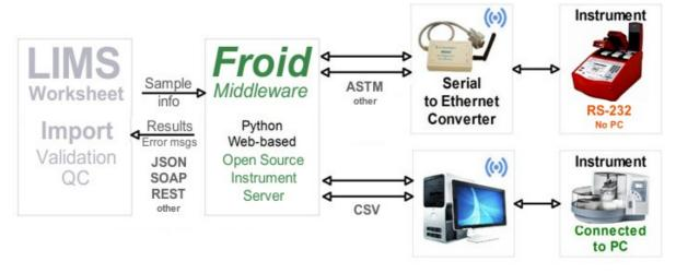
For instruments not connected to PCs and capable of serial communication only, Ethernet converters are recommended. They are not only cheaper than providing PCs for all instruments, but also don't require cabling if Wi-Fi with secure encryption is chosen.
